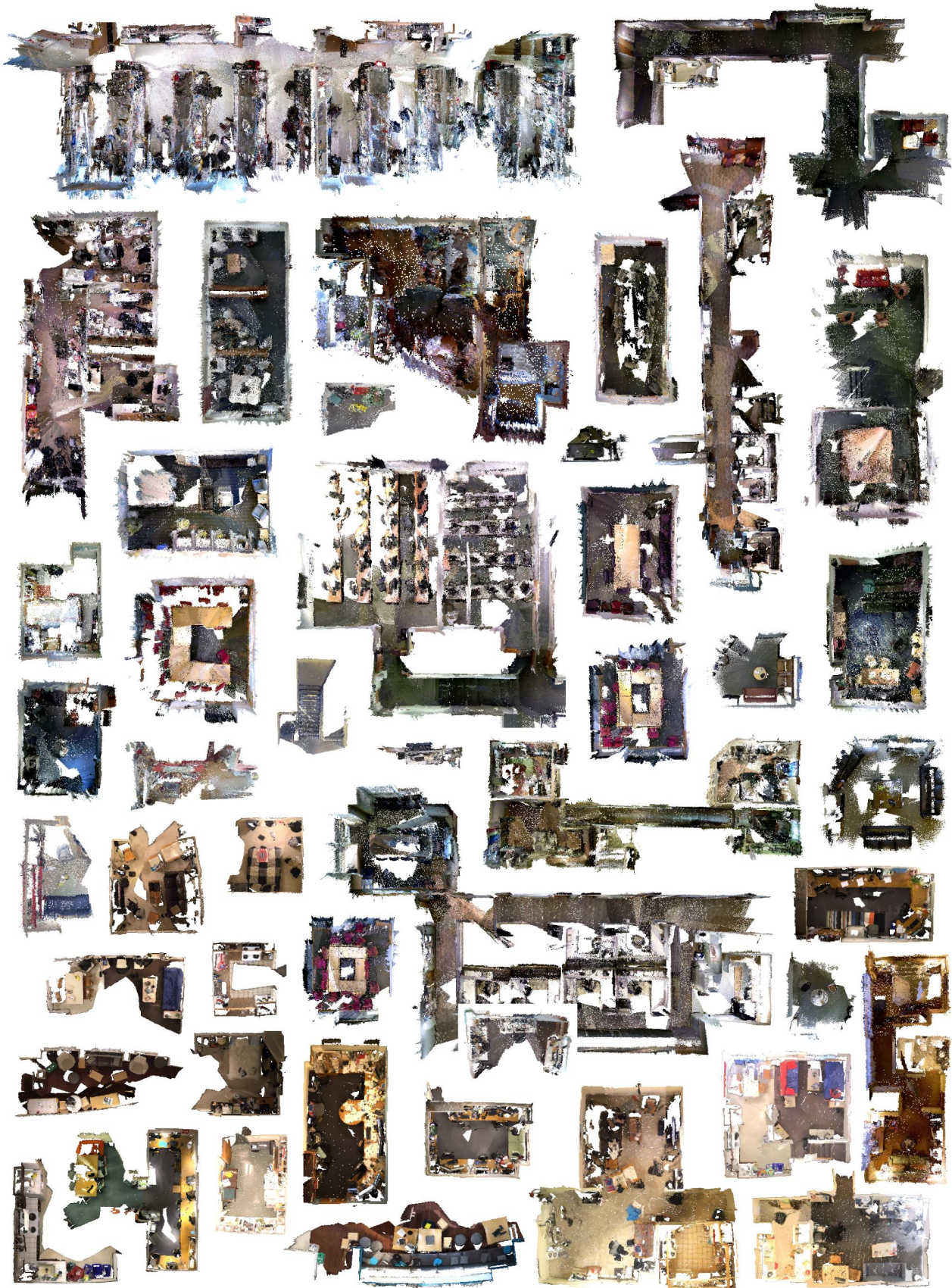
Figure 11. Visualizing several RGB-D reconstructions of the datasets used to train 3DMatch in our experiments. Each dataset contains depth scans of different environments with different local geometries at varying scales, registered together by different reconstruction algorithms. These datasets provide a diverse surface correspondence training set with varying levels of sensor noise, viewpoint variance, and occlusion patterns. Color for visualization only.
